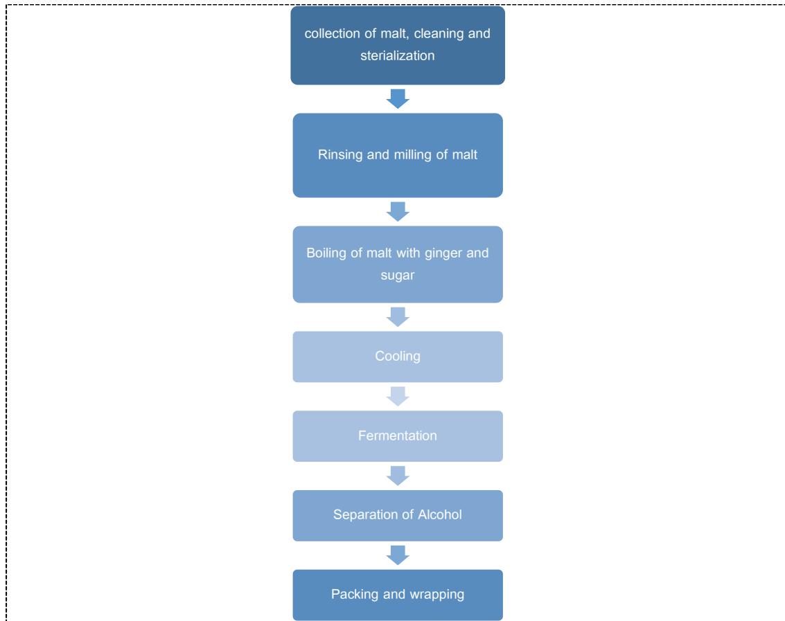
Figure 5: Production Process of alcohol-free malt beverage
